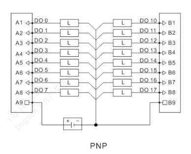
Note: The 24V power supply for A9 and B9 is provided externally.
